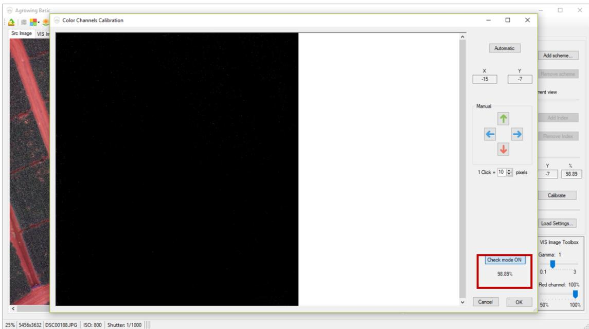
As the lenses are ~11mm apart, the digital alignment varies according to the elevation of the shooting session. The digital alignment is performed automatically whenever an image file is opened. The (X;Y) correction is also displayed on the application's main screen. In case of misalignment user can correct it manually by shifting images using arrows, when images are aligned correctly then press OK to save the results.
